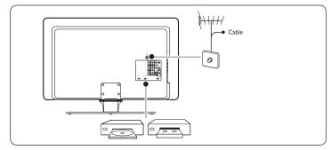
Use the TV back connectors to connect to the antenna or cable, and to permanent devices such as a high definition disc player, DVD player, or VCR.
